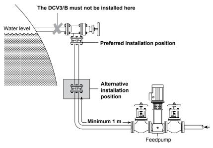
**Note:** The illustration shows preferred and alternative installations for the DCV3/B boiler feed check valve (mounted between flanges).
