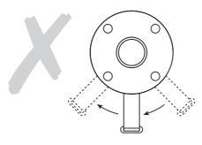
Fig. 2 Incorrect installation for liquid service
