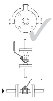
Fig. 3 Correct installation for gas service
