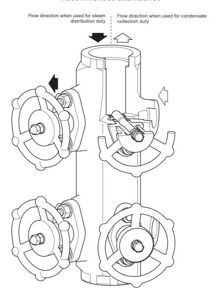
Fig. 1 Type MSC04 socket weld version shown
