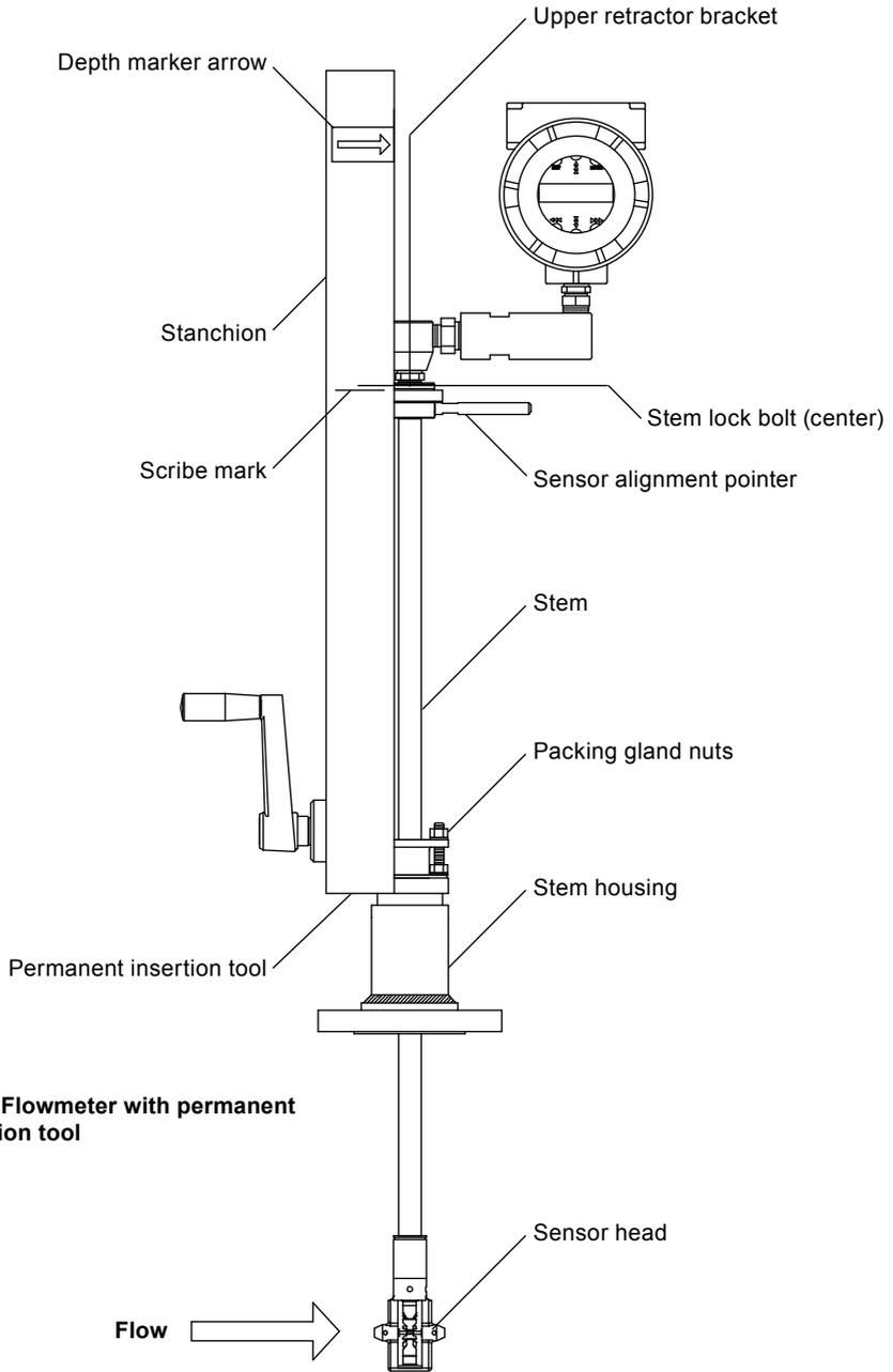
**Fig. 9** Flowmeter with permanent insertion tool
