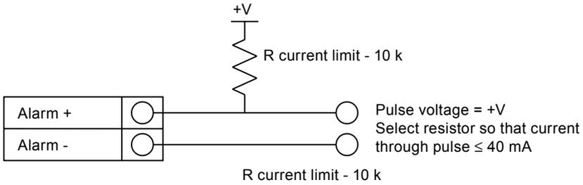
**Fig. 37 Isolated pulse output with external power supply**
