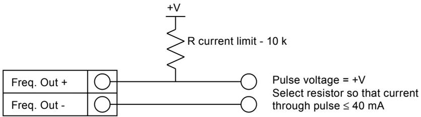
**Fig. 31 Isolated frequency output using external power supply**
