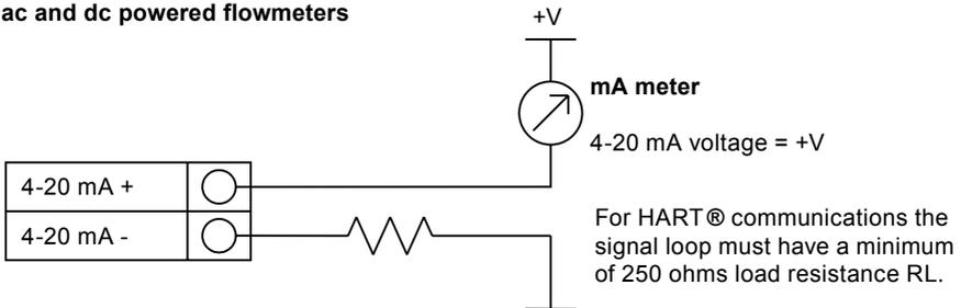
Fig. 28 Isolated 4-20 mA output with external power supply
