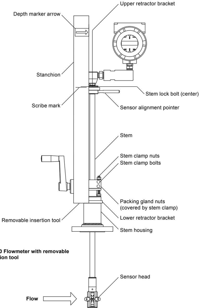
**Fig. 10 Flowmeter with removable Insertion tool**
