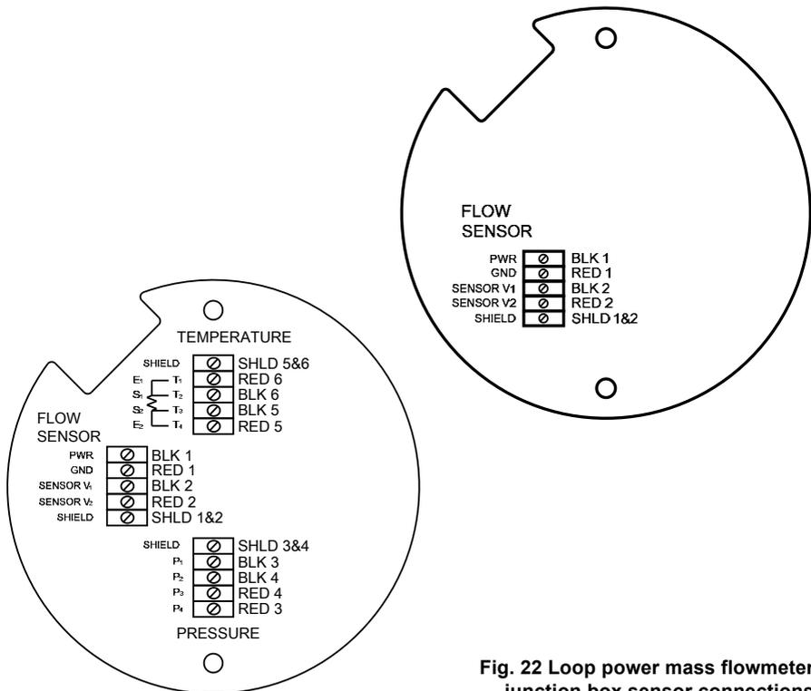
**Fig. 22 Loop power mass flowmeter junction box sensor connections**
