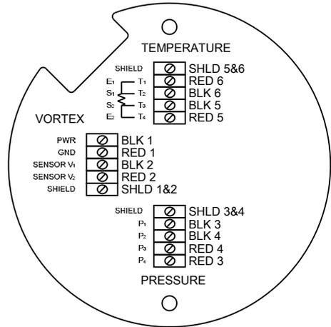
**Fig. 40 High Power flowmeter junction box sensor connections**
