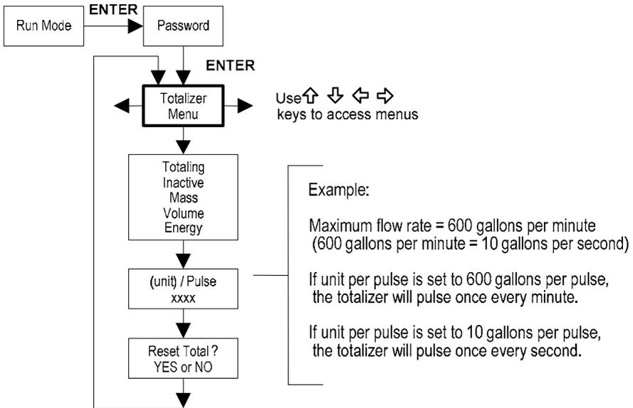
Use the Totalizer Menu to configure and monitor the totalizer. The totalizer output is a 50 millisecond (.05 second) positive pulse (relay closed for 50 milliseconds). The totalizer cannot operate faster than one pulse every 100 millisecond (0.1 second). A good rule to follow is to set the unit per pulse value equal to the maximum flow in the same units per second. This will limit the pulse to no faster than one pulse every second.
