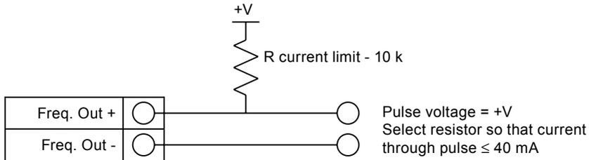
**Fig. 18 Isolated pulse output using external power**
