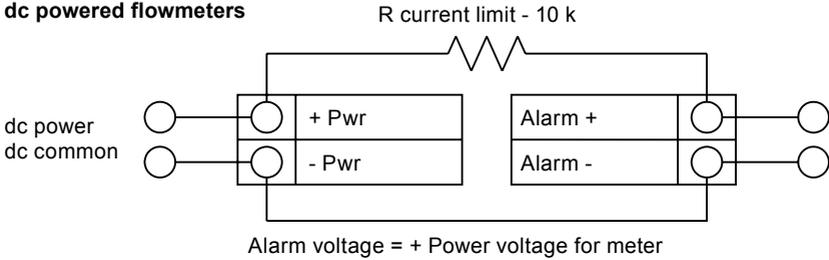
**Fig. 38 Non-isolated pulse output using input power supply**
