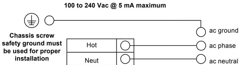
Fig. 24 ac power connections
