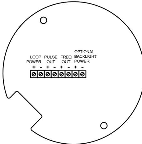
Fig. 13 Loop power wiring terminals
