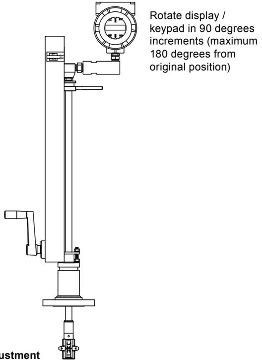
**Fig. 12 Display / keypad viewing adjustment**
