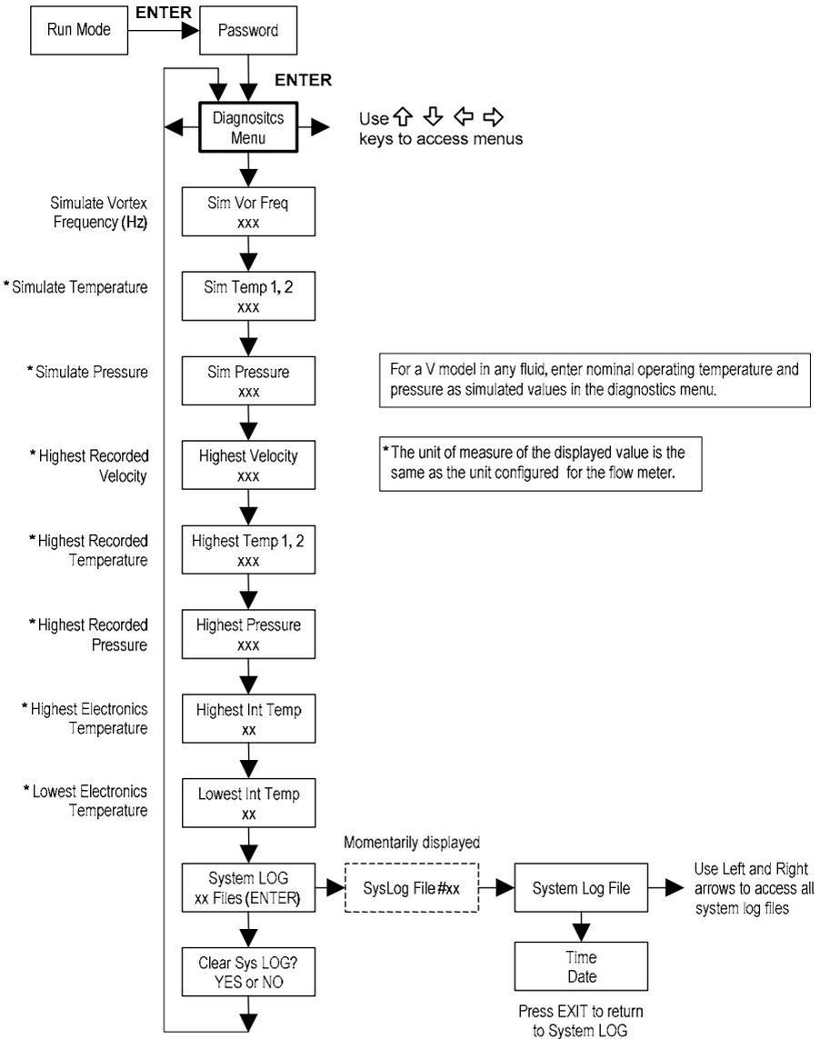
Use the Diagnostics Menu to simulate operation and review the system files. The system log files contain time/date stamped messages including: power on, power off, programming time outs, parameter faults, incorrect password entry and other various information relative to system operation and programming.
