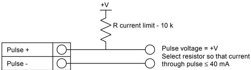
Fig. 16 Isolated pulse output using external power
