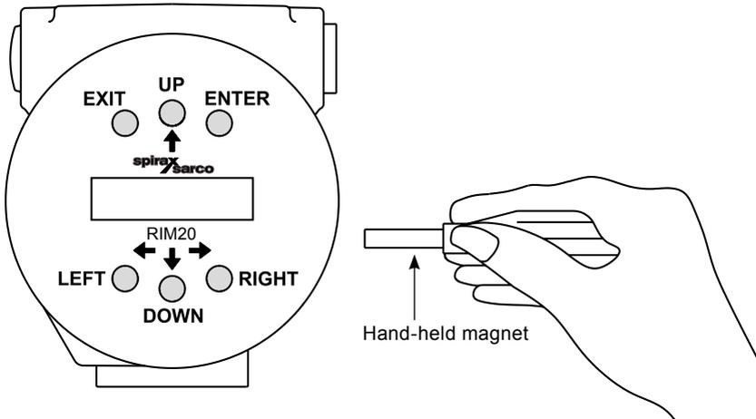
Fig. 47 Display/keypad commands
