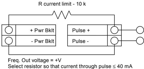
**Fig. 33 Isolated frequency output using meter provided power supply**
