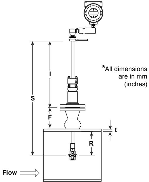
**Fig. 11 Insertion calculation (Meters without insertion tool)**
