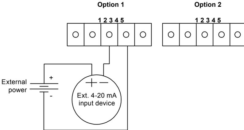
**Fig. 43 External 4-20 mA input wiring - External power supply**
