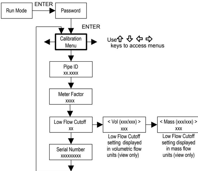
The Calibration menu contains the calibration coefficients for the flowmeter. These values should be changed only by properly trained personnel. The Low Flow Cutoff is set at the factory.
