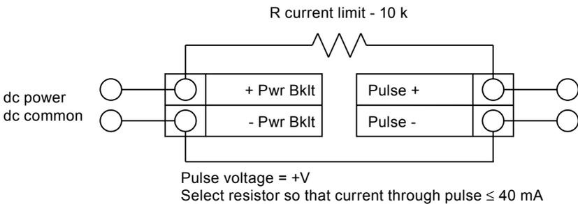
Fig. 17 Non-isolated pulse output using external power supply
