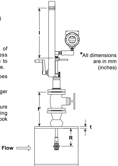
**Fig. 8 Insertion calculation (Meters with insertion tool)**
