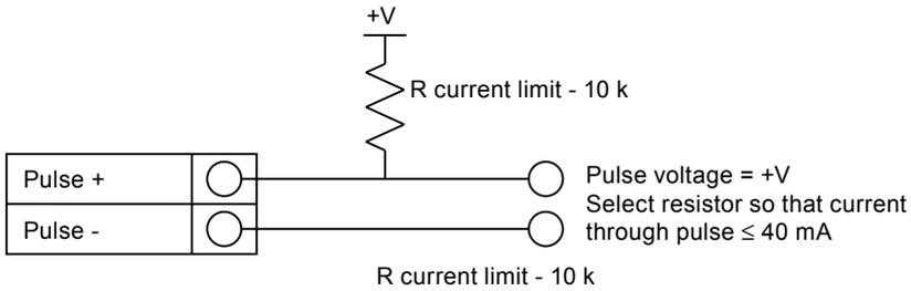
**Fig. 34 Isolated pulse output with external power supply**
