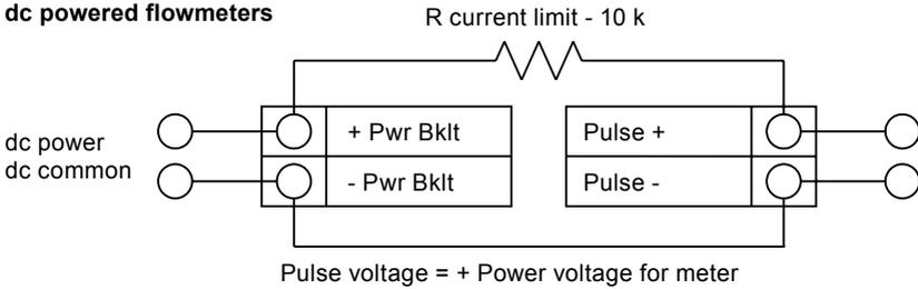
**Fig. 35 Non-isolated pulse output using input power supply**
