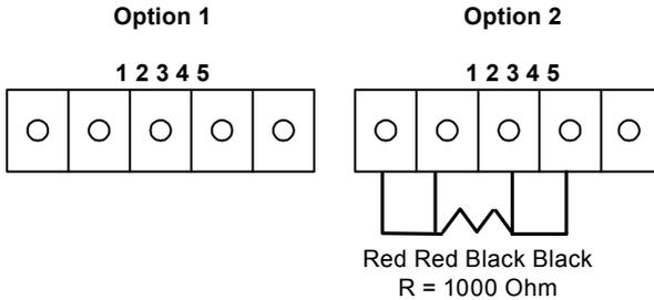
**Fig. 42 Optional energy EMS RTD input wiring**
