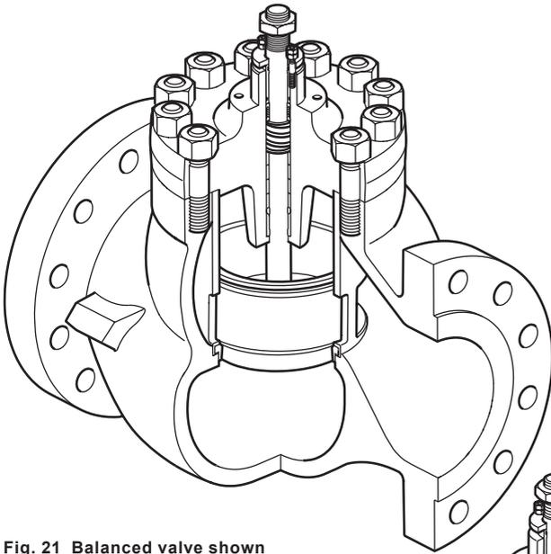
Fig. 21 Balanced valve shown
